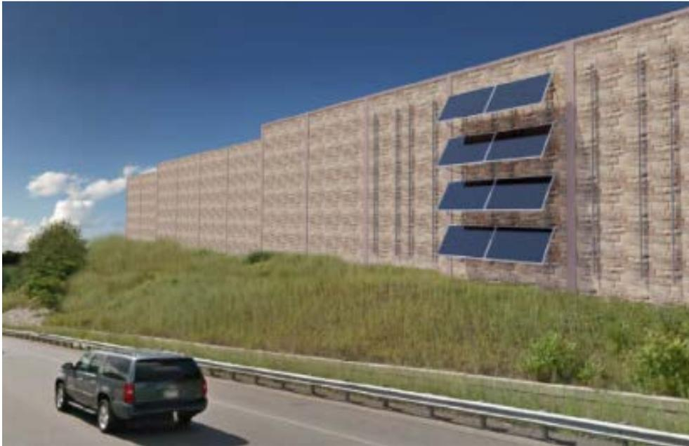
**Figure 13. Visualization of proposed configuration of solar panel retrofit on existing noise barrier in Massachusetts.**
